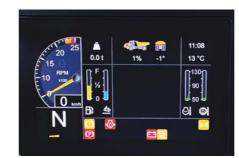
Multifunctional service and maintenance display makes it easy to check transmission oil level, plus hydraulic and electronic components.
