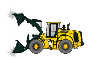
The soft end stop function reduces the hydraulic speed of the cylinder as it reaches the end of its stroke. This lessens the shock load of the stroke for increased operating comfort and better material retention.
