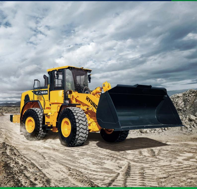
Engine Power 168 kW Bucket Capacity 2.9 - 3.3 m<sup>3</sup> Operating Weight **19450 kg**
