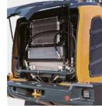
The HL970A has a dependable wide-core and fin air cooler that prevents performance degradation caused by contamination.
