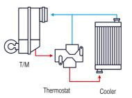
The HL970A is equipped with a **thermostat for transmission cooling**. This feature helps to warm up the fluid quickly and keeps it at the optimal working temperature, protecting components and increasing efficiency.
