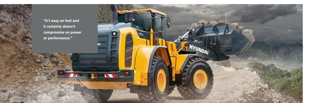
The HL970A is equipped with a **five-speed transmission and a lockup clutch**, allowing you to work more efficiently while keeping fuel consumption and emissions low.
