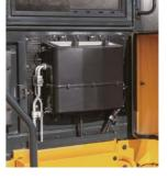
The **air conditioning filter** is easy to replace and is made from a specially selected material for superior performance.
