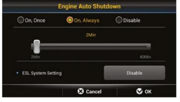
The **engine shuts down automatically when the machine is at rest** to cut fuel consumption and prevent unnecessary emissions.
