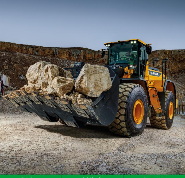
Engine Power 430 HP (321 kW) 2100 rpm **Bucket Capacity** 6.5 - 7.0 m<sup>3</sup>
